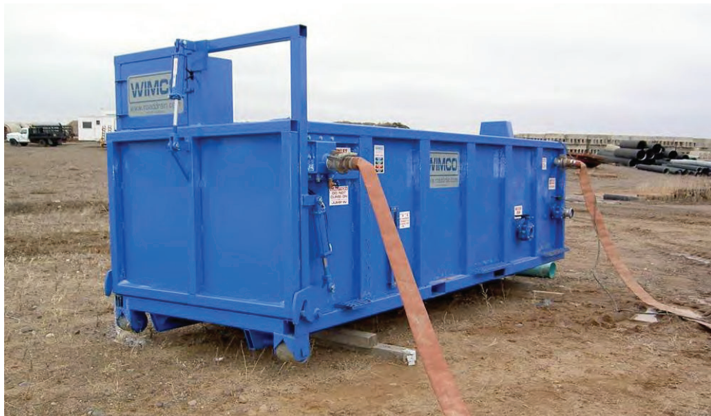
Figure 5.13: Typical sediment control system
